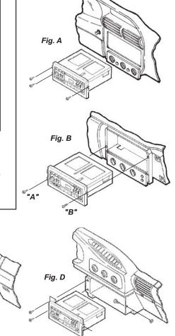
FIREBIRD 1994-99, TRANS AM 1994-99, BONNEVILLE, GRAND AM, GRAND PRIX: Reconnect the battery terminal and test the unit for proper operation. Mount the head unit/kit assembly to the sub-dash with (3) 7mm hex-head screws previously removed in step #1. (Run the upper-left screw through the dash plastic for the Grand Prix). (see Fig. A)
